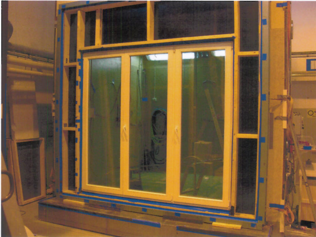
Picture 1: Inside face of the test object mounted in the frame and attached to the chamber.
