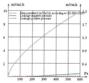
The window meets the requirements for class 4 according to SS-EN 12207 both before and after wind load
