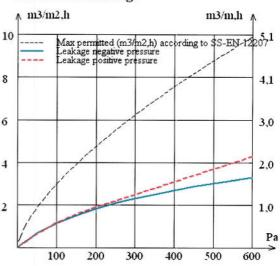
The test object meets the requirements for class 4 according to SS-EN 12207 both before and after wind loading.
